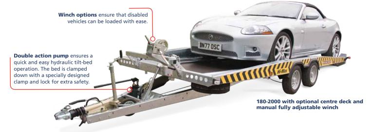
Hi-max, the Heavy Duty transporter demonstrates that with a 2,780kg maximum load capacity even the worlds heaviest mass produced cars are easily within its capabilities. With this weight on board the very low centre of gravity is important for towing safety.
