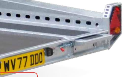
**Pull-Out Ramps** deploy in seconds and are held securely by locking pins. The ramp surface is lined in hi-grip material for safety during loading. The combination of ramps and hydraulic tilt-bed provides low loading ability, suitable for sports cars
